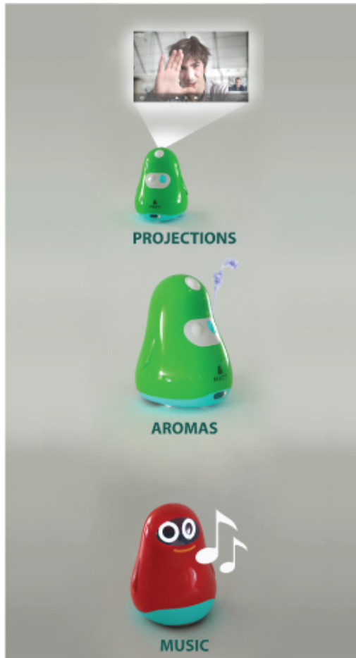
Figure 4: MATY v4: the last prototype materialized expressing examples of the multisensorial service provided to elicit the person with Alzheimer through the day
