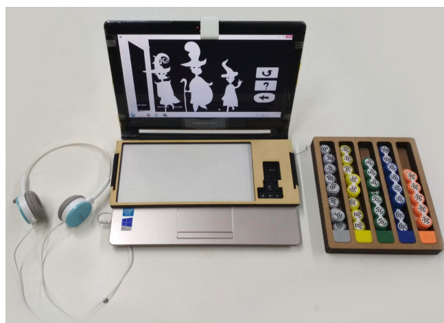
Figure 1. iCETA: headphones, computer, mirror in the camera, tangible blocks and working area on top of the keyboard.
